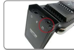
Connect a TV-Out cable to the TV-Out jack on a B4HD body.
